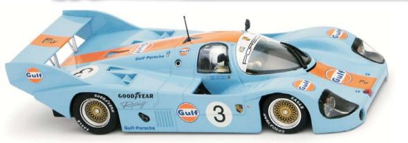
The Porsche 956 and later 962 models could be assembled with two different rear wing configurations: "low downforce", used mostly in Le Mans where the 6.5 km Hunaudières straight required a very low drag at the expense of downforce, and "high downforce", for twistier circuits.
